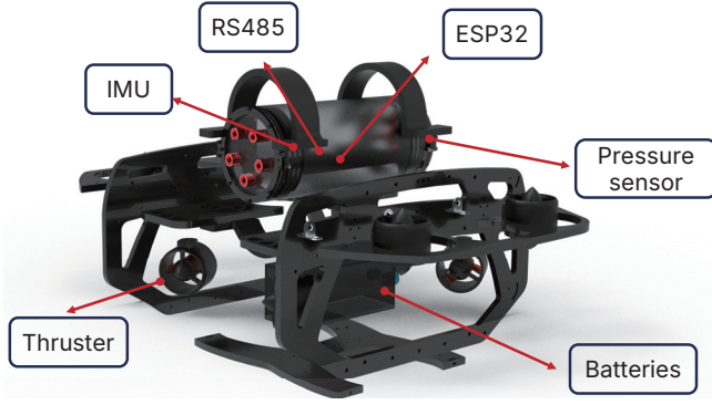
Fig. 3: Exploded view of our EasyUUV hardware platform.
